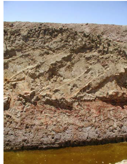
Figure 2 Typical drainage soil profile across the site
